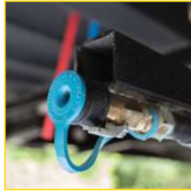
Exterior LP Connection
